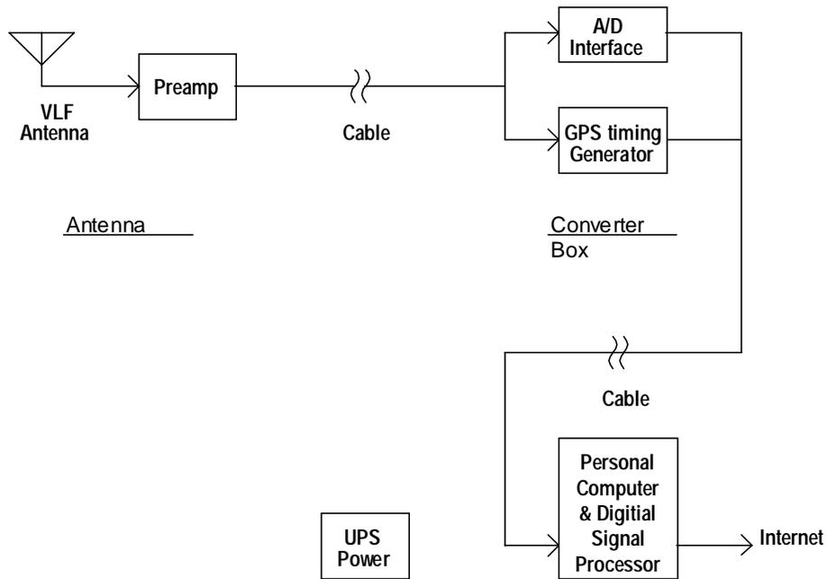
Figure 2. Sketch of ZEUS antenna receiver's component.
