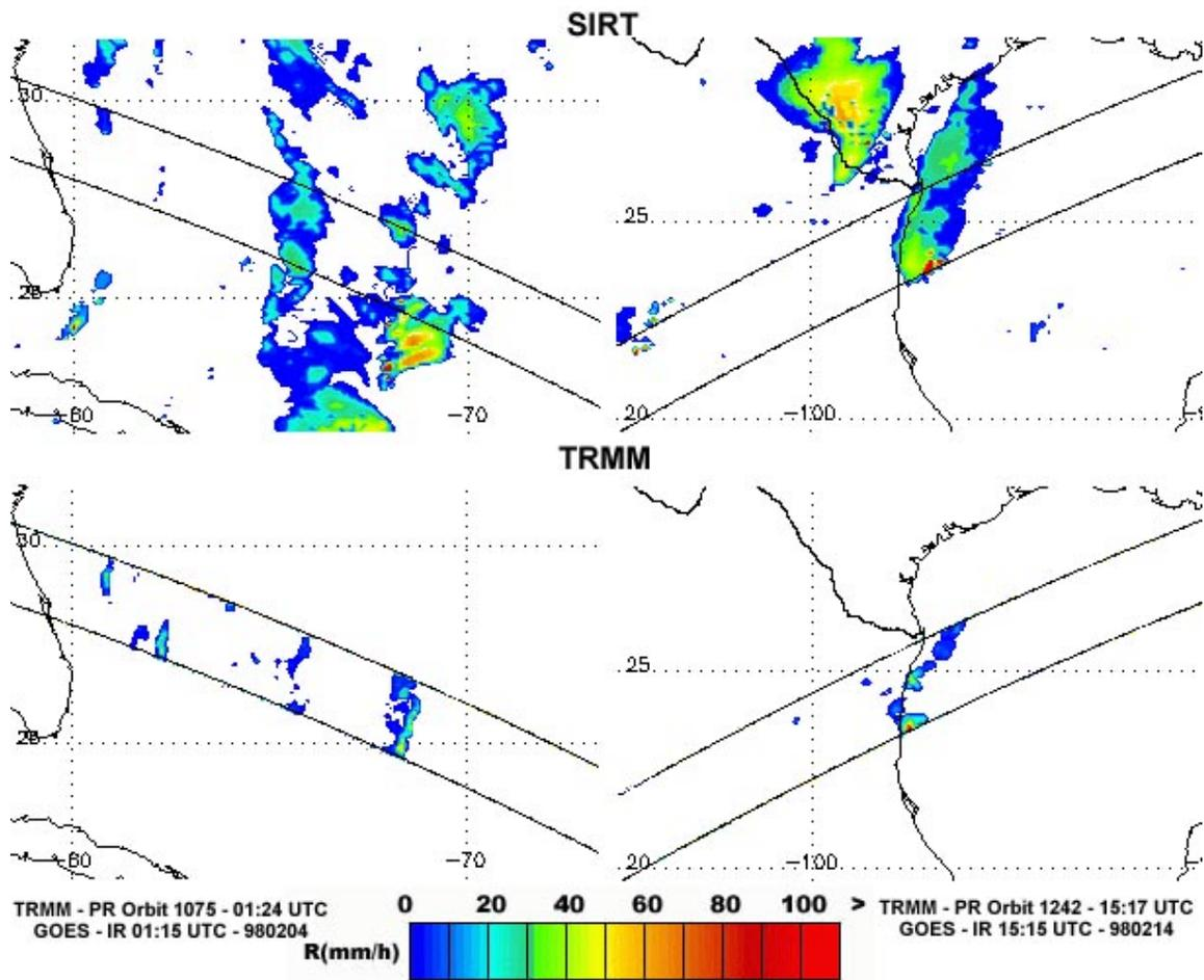
Figure 10: Instantaneous surface rainfall rates retrieved by SIRT (top panel) and TRMM-PR (bottom panel). Two storm cases are shown in this figure: (a) left, February 4<sup>th</sup> 1998 at 01:15 UTC and TRMM orbit 1075; (b) right, February 14<sup>th</sup> 1998 at 15:15 UTC and TRMM orbit 1242.
