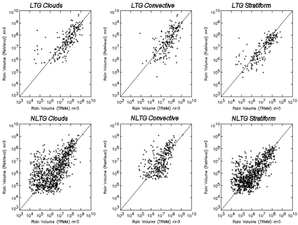
Figure 8: The same as in Figure 7 but scatter plots are for rain volumes (in cubic meter) retrieved by TRMM-PR versus SIRT.
