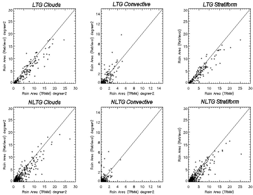
Figure 7: Scatter plots of rain area (in square degrees) retrieved by TRMM-PR versus SIRT. The top panels are for LTG clouds and the bottom represent the NLTG clouds. Total rain area is shown on the left panels, while the center and right panels show convective and stratiform rain areas, respectively.
