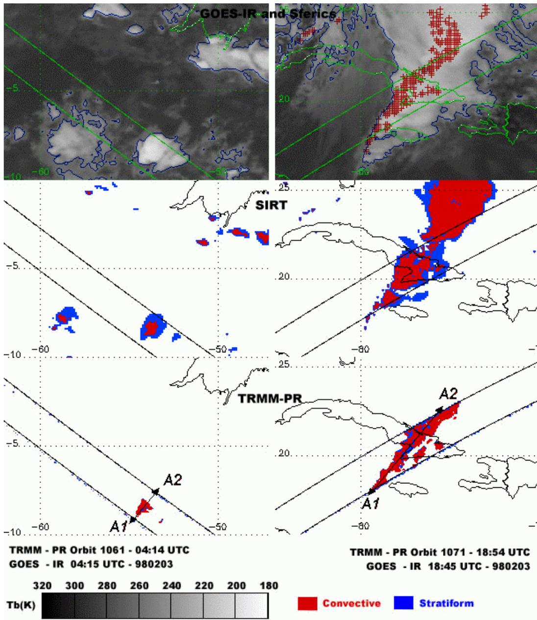
Figure 4: Top panel: GOES IR (gray scale) and lightning (red cross symbol) measurements. Middle and bottom panels show rain area retrieved by SIRT and coincident TRMM-PR overpass with the convective (red) and stratiform (blue) delineation. (a) Left column, February 3<sup>rd</sup> 1998 at 04:15 UTC and TRMM orbit 1061; (b) Right column, February 3<sup>rd</sup> 1998 at 18:45 UTC and TRMM orbit 1071
