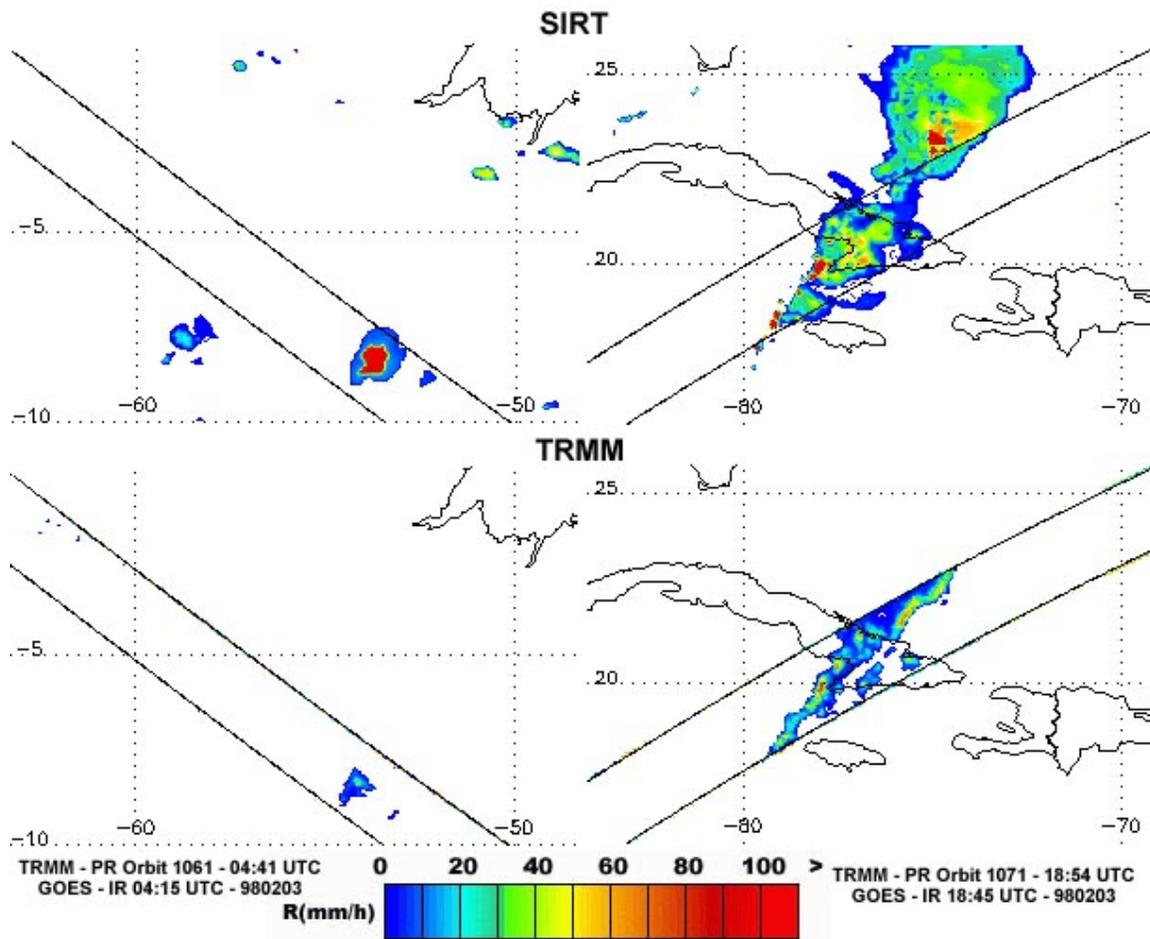
Figure 9: Instantaneous surface rainfall rates retrieved by SIRT (top panel) and TRMM-PR (bottom panel). Two storm cases are shown in this figure: (a) left, February 2<sup>nd</sup> 1998 at 04:15 UTC and TRMM orbit 1061; (b) right, February 2<sup>nd</sup> 1998 at 18:45 UTC and TRMM orbit 1071.
