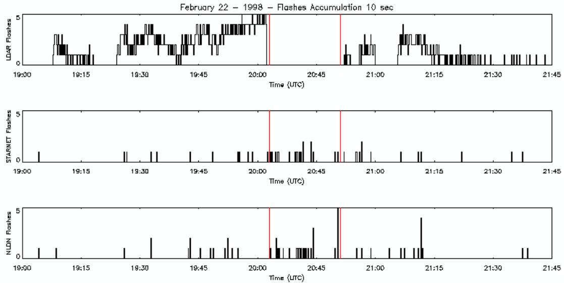
Figure 10. Time series of total flashes accumulated on 10-second intervals observed on February 22<sup>nd</sup> 1998 (19:00 UTC through 21:45 UTC) by LDAR (top), STARNET (center), and NLDN (bottom). Note that during 20:02-20:52 there were no available LDAR data (red bars) (The 20:45 UTC time also coincides with 20:15 UTC).
