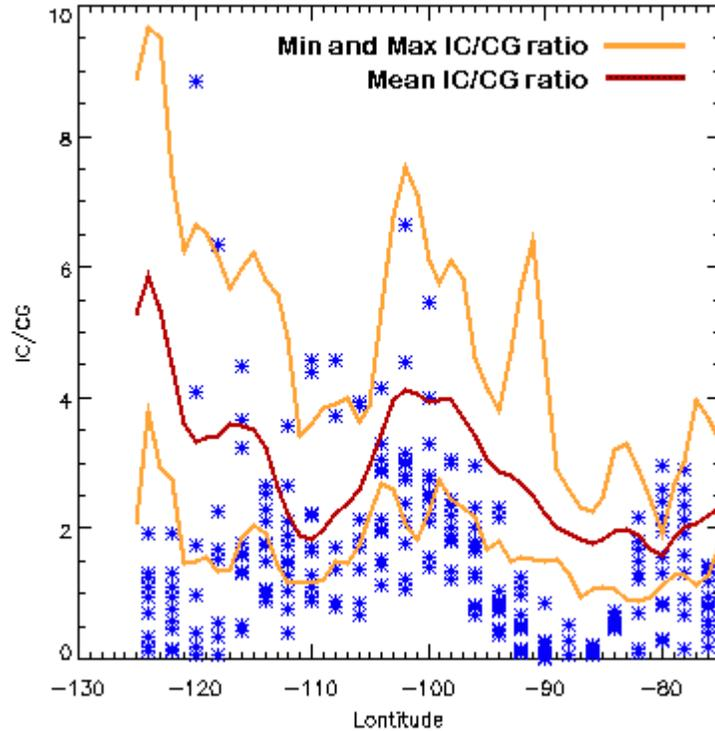
Figure 12: Mean IC:CG ratio values for hourly intervals over 2 degree longitude zones for the period of December, 1997 through February 1998 (blue asterisks). Red and yellow lines represent mean and maximum/minimum values of IC:CG OTD/NLDN ratios evaluated by Boccippio et al. (2001c).
