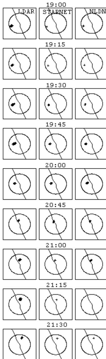
Figure 9. Spatial distribution of observed LDAR (left), STARNET (center) and NLDN (right) flashes at 15-minute intervals. The circle radius is 100 km and the center is at LDAR central station.
