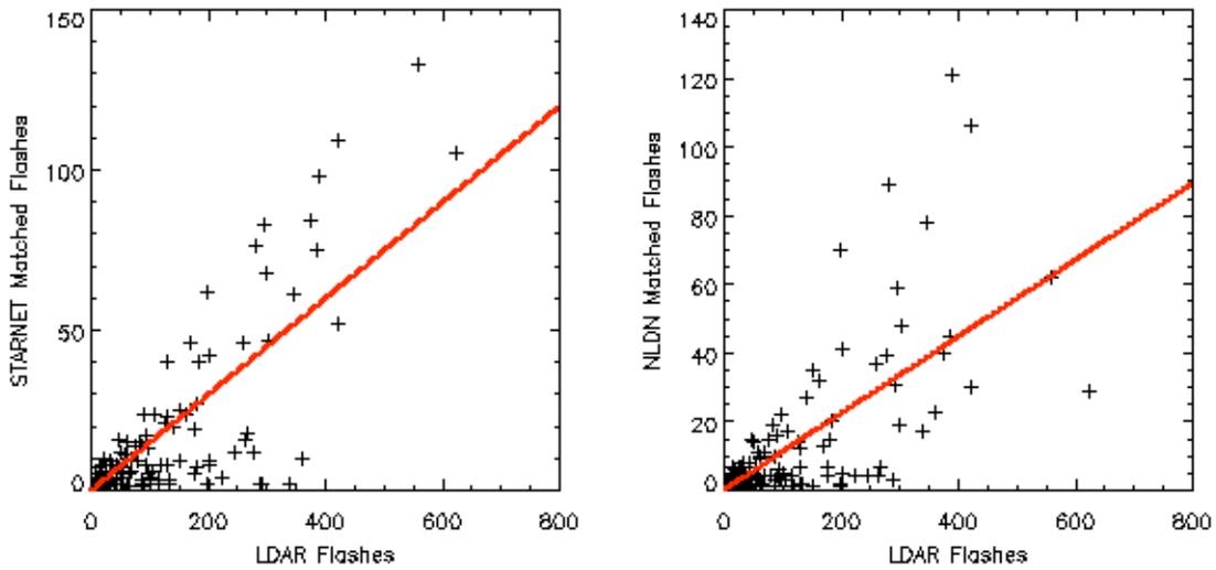
Figure 7. LDAR total lightning flashes versus total STARNET (left panel) and NLDN (right panel) matched flashes for each of the 301 selected 15-minute storm cases. The red lines represent the least-square fit of the above data set.
