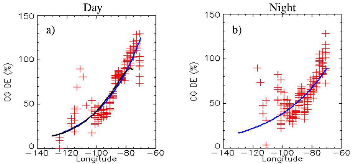
Figure 2: Sferics cloud-to-ground detection efficiency during the daytime (a) and nighttime (b) period for a timing window of 100 ms, and 50 km space window. The blue line represents the best fit of DE determined as a function of longitude. The black line is the DE determined from equation (1).
