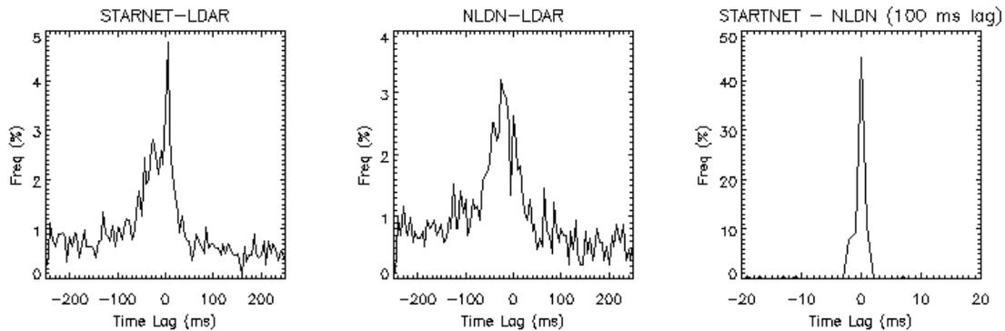
Figure 6. Time lag distribution of LDAR vs. STARNET matches (left panel), NLDN vs. LDAR matches (center panel), and STARNET vs. NLDN matches (right panel). Negative time lags represent time delay with respect to LDAR (left two panels), or STARNET to NLDN (right most panel), while positive is the contrary.
