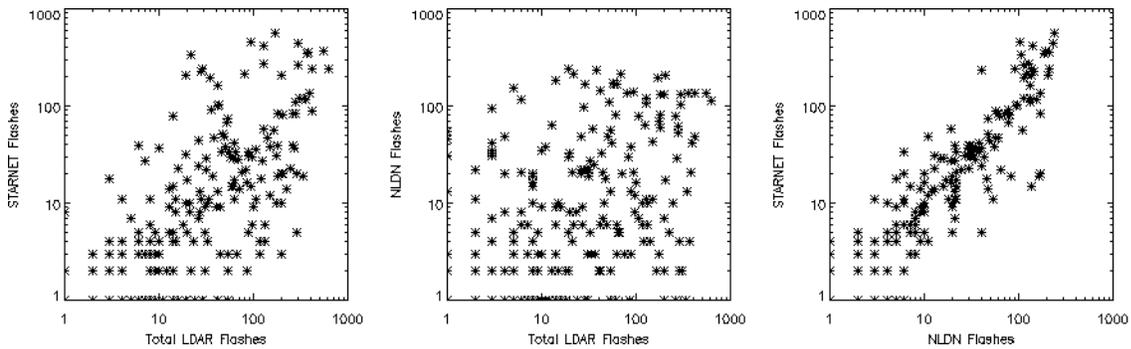
Figure 8. LDAR versus STARNET (left panel) and NLDN (middle panel) total flashes within the 15-minute storm intervals; Right panel, NLDN versus STARNET total flashes.
