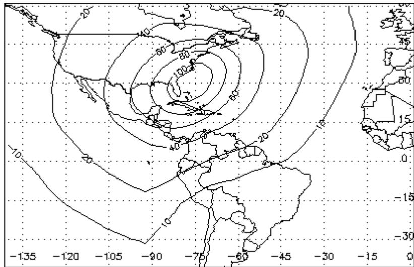
Figure 4. Daytime STARNET's CG DE spatial distribution evaluated using the theoretical signal strength model adjusted by the experimentally derived CG DE values.
